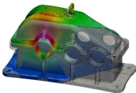
Steady or transient finite element analysis using e.g. volumes, shells, beams, prestressed bolts, glued joints and/or contact with **Code\_Aster**.
