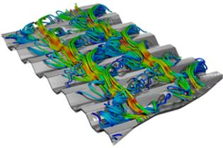
Optimization of **heat exchangers** for maximum heat transfer at minimum pressure loss by application of structured surfaces.
