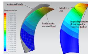
**Fluid/structure interaction** by coupling FEM and CFD analyses.
