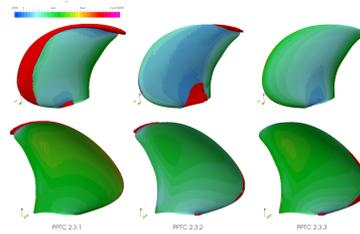
Analysis of **cavitation** at marine propeller blades and other devices operating in liquids.
