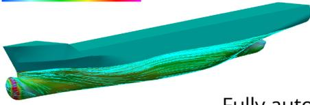
Fully automated computation of **ship resistance** computation using CFD methods. Optionally including trim and sinkage.
